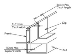
Fig. 8 Mounting requirements for rails overlapping the short-side frame
