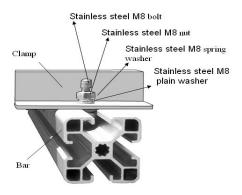
Fig. 8 Schematic diagram of the fringe clamp
