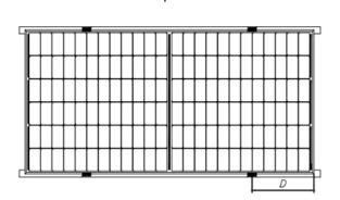
Fig.3 Rails overlapping the long-side frame
