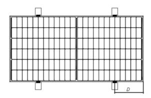
Fig. 4 Rails vertical to the long-side frame
