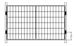
Fig. 5 Rails overlapping the short-side frame
