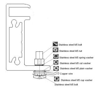
Fig. 18 Grounding the aluminum frame with copper wire
